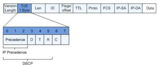
O to 2 bits are Precedence fields representing the 8 priorities of message transmission ranging from 7 to 0 from high to low, with either Level 7 or 6 as the highest priority that is generally reserved for routing or updating network control communication. User-level applications only have access to Level O to 5.
